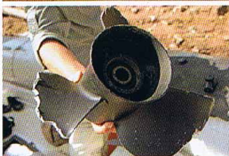
Above: The all too common damaged prop. Others: Negotiating the Khone falls and rapids with craned assistance
